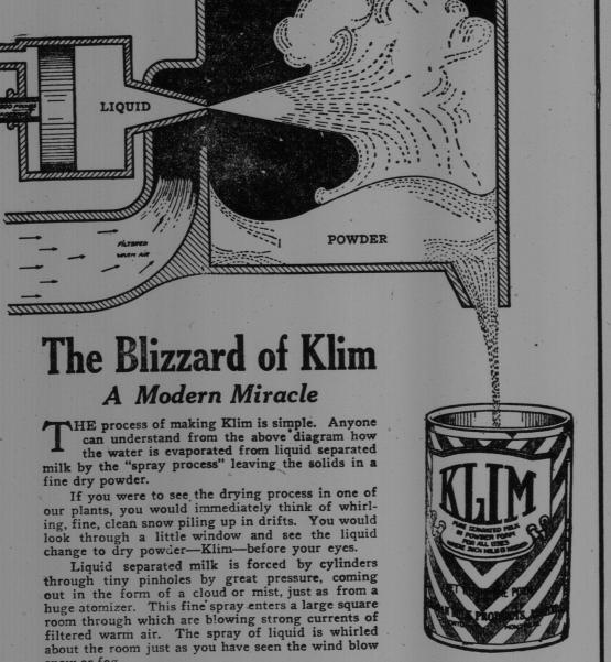
The warm air immediately absorbs the moisture from the spray and the solids settle to the floor in white drifts of Klim. The moisture-laden air passes out through screens which prevent any of the Klim from escaping.
