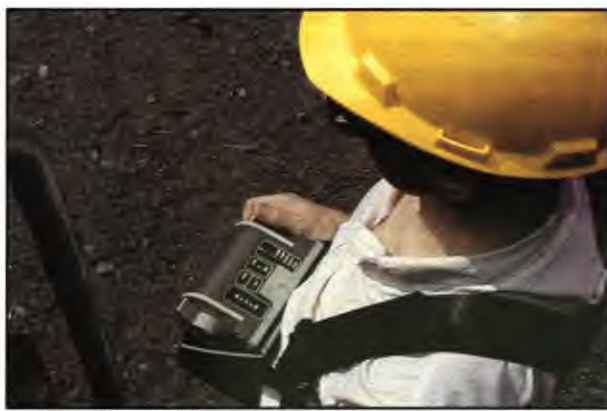
All locomotive controls required by operator are available on portable Beltpack®
