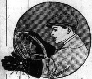
HERE'S a new kind of Motoring Glove that is very useful for motorists and auto delivery men at night for finding street numbers, locating trouble on car, etc., and for giving hand signals while driving. The tiny electric bulb on the back is ingeniously connected with a small battery inside the lining. By simply pressing thumb against first finger a connection is made and incidentally a brilliant ray of light. The bulb and battery are detachable when gloves are worn in daytime.
