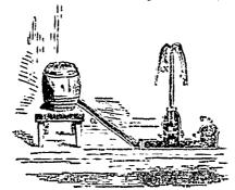
as it cannot escape through (r), it opens the valve in in the ram, and rushes up the pipe (x). The mometum ceases, and (s) again opens, when the same action is repeated. So apa is the action of the machine that the valve (s) is in continual vibration, and an incessant stream of water is produced. See pages 15 end 307 of the Canada Paimer of last year.
