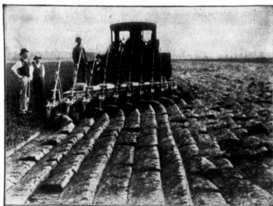
Rear View of an Avery Plowing Outfit consisting of an Avery 22 H.P. Double Undermounted Engine and 10-Gang Plow Attachment.
