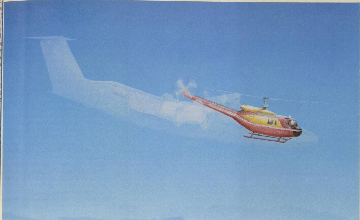
The NAE Bell 205A-1 helicopter, modified for use as an airborne V/STOL aircraft simulator, is a powerful research tool for investigating the handling qualities and control problems of hypothetical and new aircraft. It was flown in support of augmentor wing, engine-failure flight tests and it has also provided control design data for aircraft such as the DHC Dash 7. (Graphic: John Bianchi)
