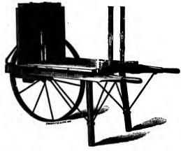
HIS cut represents our IMPROVED HACK BARROW, adapted for brick and tile. The rake in front is used for wheeling tile, and is lifted out when being used for brick. The wheel is the same as in the Platform Barrow, The Barrow is well braced and framed together, and has been tested with ninety brick, weighing seven pounds each, which is the amount usually wheeled on this style of barrow.
