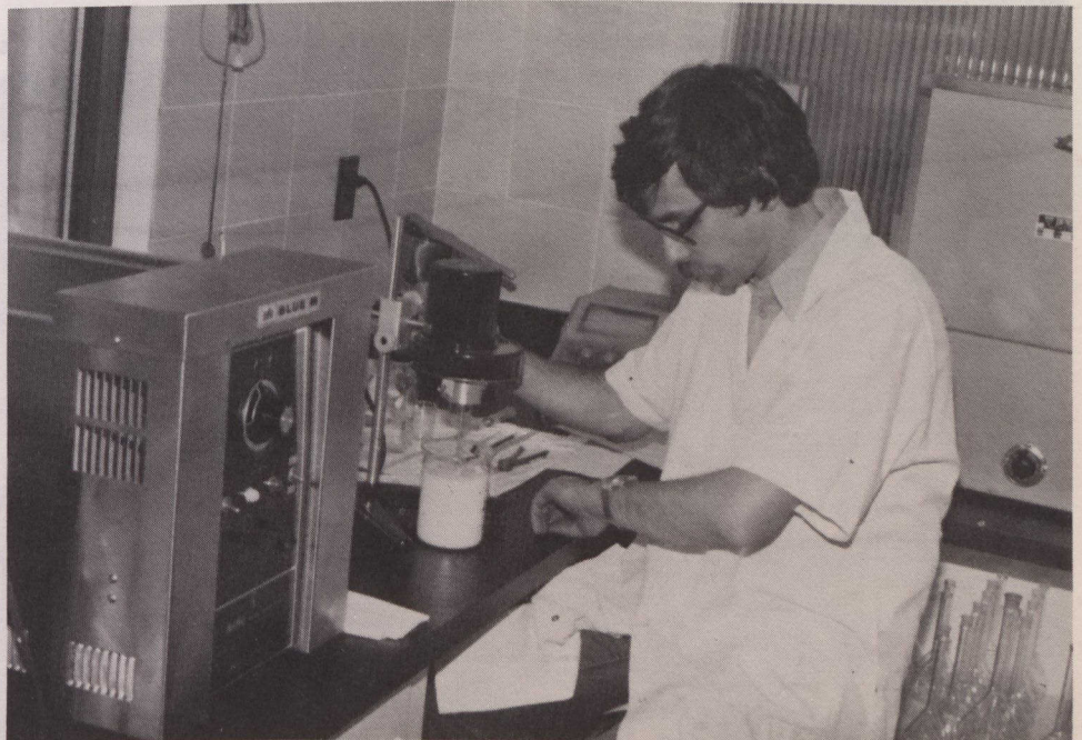
Development of a fortified skim milk sterilized by the ultra high temperature system with added milk proteins and vitamins, has been completed. Dairy employee Lester Dobosz measures the viscosity of the finished product.
