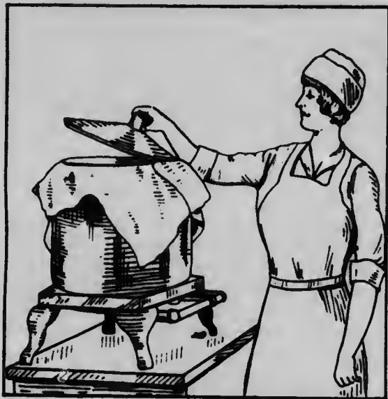
Fig. 2. Adjustment of ordinary cover with cloth gives a tight fit and boiler will hold the steam.
