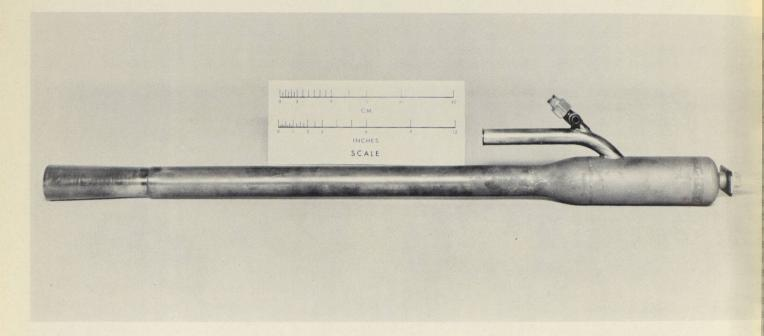
The hot products of combustion are discharged from the pulse jet into a venturi when they are mixed with secondary air and cooled to an acceptable temperature of 190 to 225 degrees Fahrenheit. If higher temperatures are used there is a danger of setting the wooden ties under the switch on fire.
