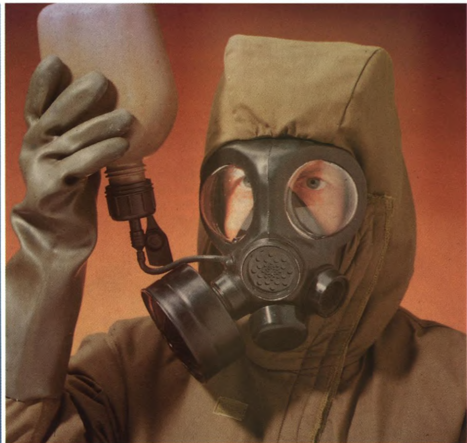
The C4 mask fits snugly under hood of CW protective clothing.
