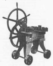
stead of levers. This wheel turns a small pinion which meshes with a large gear, making the machine very powerful. One man on the wheel can easily upset a tire  $7 \times 1 \frac{14}{3}$  inches or an axle  $3\frac{16}{3} \times 3\frac{16}{3}$  inches. The frame is of heavy cast-iron. The machine is mounted on cast-iron wheels, so that it can be easily shifted about the shop. This tire upsetter weighs complete about 900 pounds.
