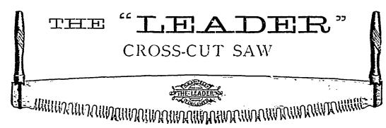
These Saws are made from the best Double REFINED SILVER STEEL, warranted four gauges this ner on back than front, and the only Saws on the market that are a perfect taper from the points of the teeth to the back, and require less Set than any other Cross-Cut Saw.
