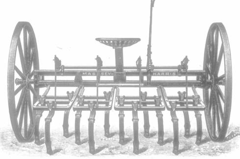
The Tooth Seat is adjustable for spacing the teeth to suit different kinds of cultivating. Equipped with 7 1/2" weeder blades, it makes a very effective implement for cleaning up weeds.
