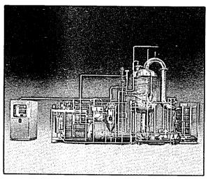
TCI-Superior, together with Chemetron Inc. of Louisville, Kentucky, undertook the design, manufacture, supply and installation of a system to concentrate and aseptically process yogurt fruit topping.
