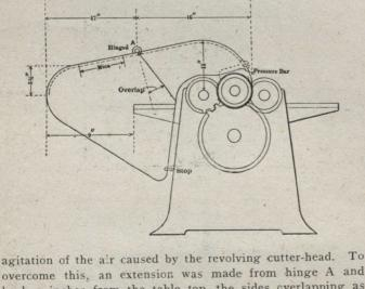
agitation of the air caused by the revolving cutter-field. For overcome this, an extension was made from hinge A and back 9 inches from the table top, the sides overlapping as shown. The top rounding down about 3½ inches left about 3 inches between top of table and bottom of this rounded edge. Through the top was cut an opening about 6 by 14 inches and in this was fastened a piece of mica such as is used for automobile shields; this made it possible to see the work as it came through the planer.
