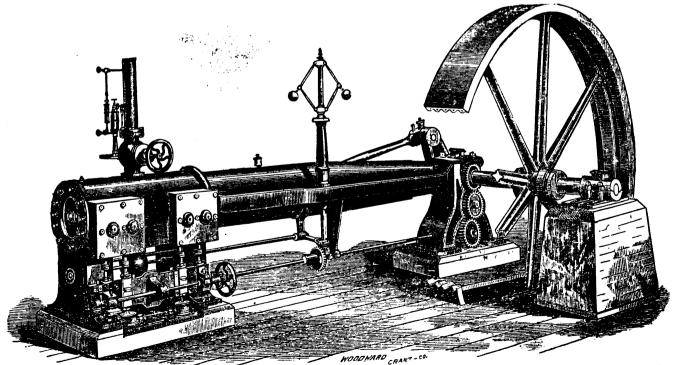
The above Cut shows our Improved Variable Cut Off Engine, which combines Economy and simplicity in a higher degree than any other Engine now in use. All material and workmanship warranted. A Patent has been applied for. Send for Circular. Steam Eugines and Boilers, Flouring and Saw Mills, Millstones; Wood working and Stave and Barrel Machinery, Wool Machinery, Flax
