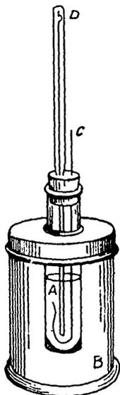
It consists of an outer jar, B, in which the freezing mixture of ice and salt is placed. Suspended in the jar is the tube, A, and projecting into this is a wire stirring-rod, C, and a thermometer, D. This thermometer is graduated in one-hundredths of a degree centigrade, usually from one degree above to four degrees below zero. The scale is sufficiently coarse to allow of the reading of 1/200 of a degree.
