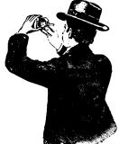
THE accompanying illustration shows an operator taking vertical angles with the Brunton Patent Pocket Transit.
