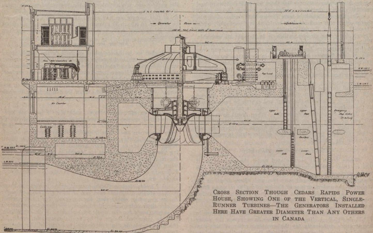
CROSS SECTION THROUGH CEDARS RAPIDS POWER HOUSE, SHOWING ONE OF THE VERTICAL, SINGLE-RUNNER TURBINES—THE GENERATORS INSTALLED HERE HAVE GREATER DIAMETER THAN ANY OTHERS IN CANADA
