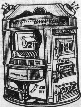
Sectional View of Buck's Leader Furnace
