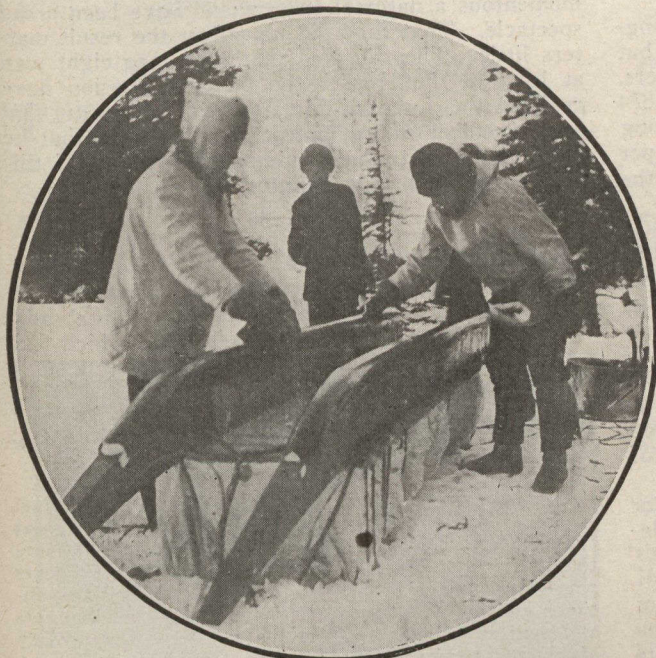
Glazing a Sub-Arctic Sled-shoe With a Veneer of Ice.
