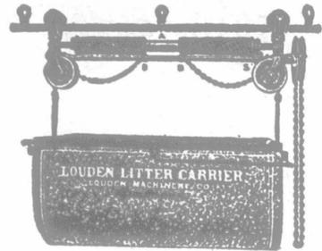
The hoisting gear is simple and very easily operated. The box is raised and lowered by means of an endless chain working on a screw gear. By pulling the chain one way the box is raised, while by pulling in the opposite direction it is lowered.
