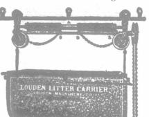
The hoisting gear is simple and very easily operated. The box is raised and lowe ed by means of an endless chain working on a screw gear. By pulling the chain one way the box is raised, while by pulling in the opposite direction it is lowered.
