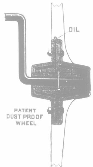
it; oil cannot leak out of it; and the axles cannot spring nor weaken a little bit. Once oiled these wheels run silently and perfectly for days—another light-draft feature gained by reducing friction. Send for details of this practical device—it will pay you.
