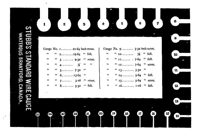
Compare your circular and gang saws with the above gauge, and estimate the amount you would save each season. By cutting your stock with 14-15 or 16 gauge Band Saw—either gauge thoroughly practical. The Band will cut 1-8th —say 7-64. Your circular, if 6 gauge, will probably cut 21-64. The saving is enormous. You cannot afford to continue the waste.
