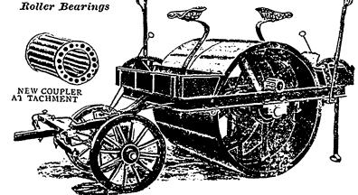
With Roller Bearings and New Patent Coupler Attachment, either 21/4, 31/4, 41/4 or 51/4 tons. All one size frame, drum, and width of tread and can be extra weighed 2 tons each. Address for Catalogue
