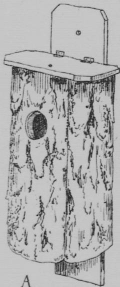
Fig. 1 Nesting Box Made of Slab-wood. Ready for Hanging.
