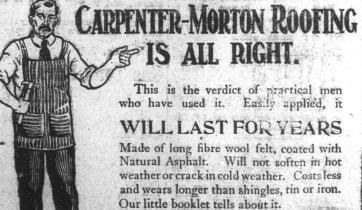
who have used it. Easily applied, it WILL LAST FOR YEARS Made of long fibre wool felt, coated with Natural Asphalt. Will not soften in hot
