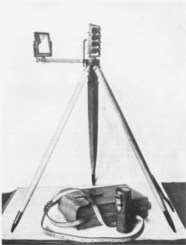
Fig. 102 Forest Service type of heliograph, one-mirror
