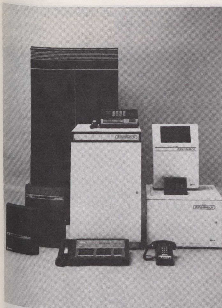
Mitel Corporation, a leader in Canadian telecommunications, produces telephone equipment such as the Superswitch Family shown here. The line runs from the SX-5, with six extensions and two trunks to the SX-2000, a digital switch with capability of over 10,000 lines.
