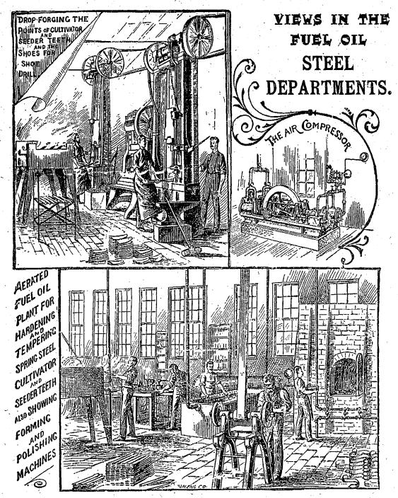
This new process of manufacturing Spring Steel Teeth produces a finer grade of teeth than otherwise possible. The Fuel Oil is atomized into the furnaces and ovens under high air pressure and creates a remarkably regular, even heat, which results in the hardening and tempering of the steel teeth being perfectly performed, and without any burning or injury to the steel.
