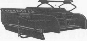
Loose earth, sand, gravel, lime or any other commodity of like nature can be dumped in one pile, or spread along as desired. The contrivance for dumping is operated by foot, so the driver has the use of both hands. Load can be dumped without driver leaving the seat, and the bottom can be drawn up into position while start-
