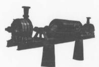
Two Worthington 3 stage Turbines and McCormick Water Wheels, built for Port Arthur, Ontario, Water Works. Combined capacity 1440 gallons per minute against 350
