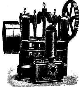
We illustrate in this advertisement a typical Pump for Mine Work. This is our Triplex Power Pump, fitted with tight and loose pulleys as shown in cut. It is the regular Triplex type with the three cranks 120 degrees apart; crankshaft and connecting rods are of steel; gears machine-cut from the solid; plungers of brass and all details carefully worked out. This Pump is especially adapted for service with Electricity as the motor power.
