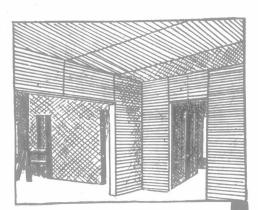
Bishopric Sheathing Board is a combination of lath, asphaltmastic and heavy, rosin sized, high-grade cardboard. Walls and ceilings made of "Bishopric" are satisfactory in every way and your house will be warm in winter and cool in summer because the Asphalt-Mastic is absolutely moisture and temperature proof.
