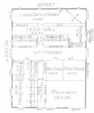
It is not necessary to have all the loose cattle together, as gates can be swung on the outside wall at the posts, or fastened in the cement, and swung along the wall as desired. If the barn were two het lenger, it would probably be better
