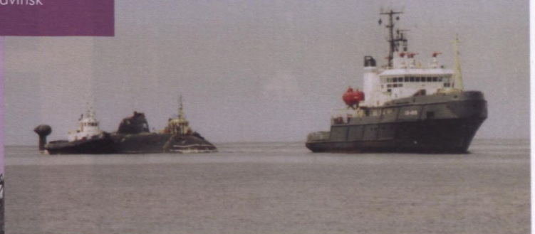
Decommissioned submarine being towed to the Zvezdochka shipyard by main and auxiliary tug boats
