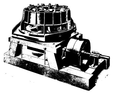
This mill is largely used for crushing ores that are not too hard and sharp. It is also extensively used for re-grinding middlings and tailings in concentration mills. One mill alone has 40 HUNTINGTONS for this purpose.
