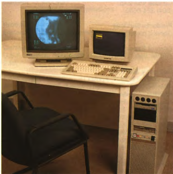
The Optical Memory Subsystem workstation produced by ALI Technologies Ltd. reviews and enhances digital images, and stores the images on optical disk.
