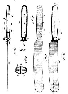
and then plugging said vent opening, substantially as set forth. 3rd. As a new article of manufacture, an article of table cutlery having a blade and flat tang formed integral, and a handle and bolster portion formed of sheet-metal scales fitting against opposite sides of the blade and housing and contacting with the edges of the tang, all the parts being secured together and the joints between them hermetically sealed with molten metal, substantially as described.
