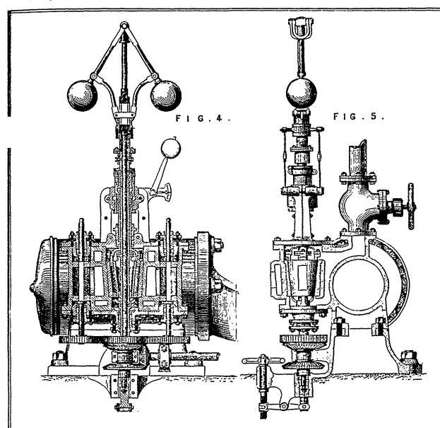
HORIZONTAL ENGINE WITH RADINGER'S VALVE GEAB.
