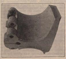
Fig. 37. Cast Steel Segment.
