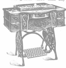
The Sewing Head forms the reliable and time-tested double-lock stitch, extremely high arm, well equipped with improvements and labor - saving devices. Improved disc tension, with automatic release. Steel forged, double width, positive four-motion feed. Improved automatic stitch regulator on face of arm. Automatic bobbin winder. Positive cam-driven take-up. Gear - releasing device. Self-threading shuttle. Oil hardened steel working parts.
