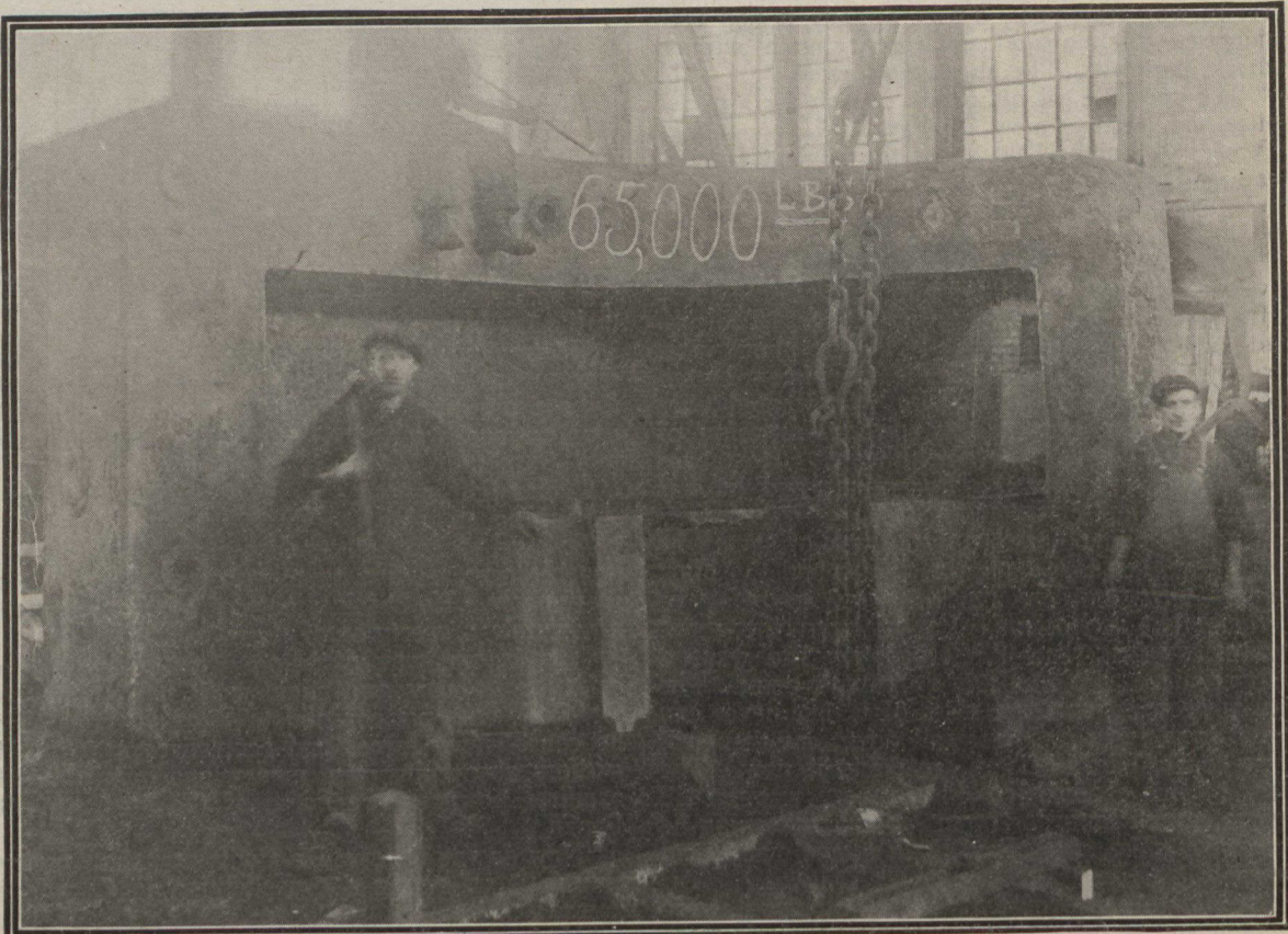
32½ Tons of Iron in a Single Casting for a Rolling-mill Engine; Produced at the International Engineering Works, Amherst, N.S.
