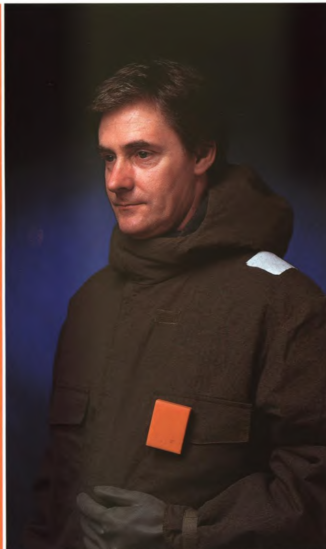
The Badge dosimeter measures gamma and, optionally, neutron doses.
