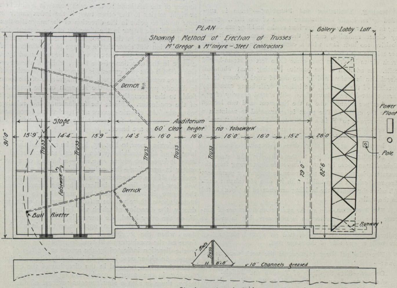
securely bolted to skids as shown in the sketch, and were then moved by hand tackle along greased channels to their own anchor bolts. Owing to the great span each auditorium
