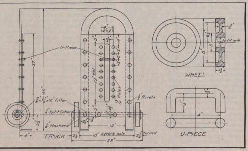
Cylinder Head Truck for Fitting Heads without a Crane.
