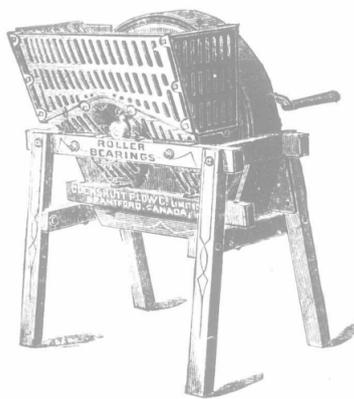
**Turn Crank One Way and it Slices—Reverse Crank and it Pulps Roots**
