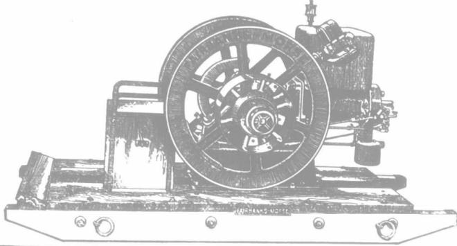
Horizontal Evaporator Tank Engine mounted on skids.
